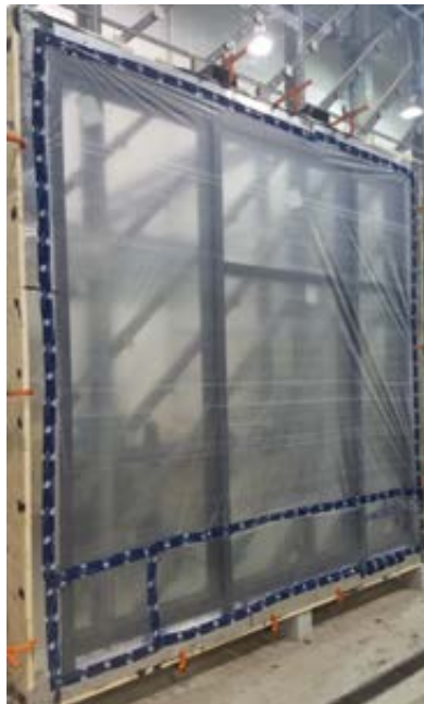
MC Wall – Façade window wall system – Exterior
